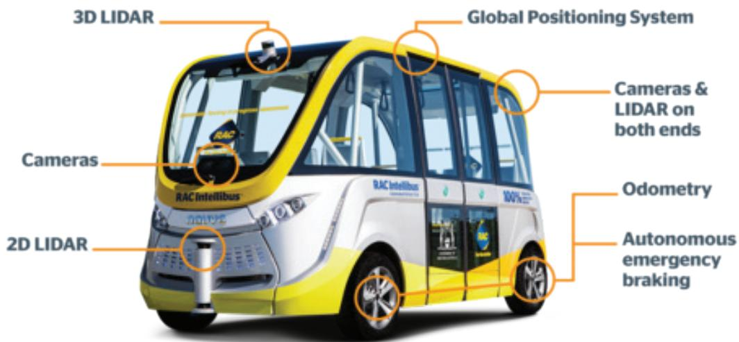
Image source: <http://www.caradvice.com.au/476314/australias-first-autonomous-bus-hits-the-road-in-perth/>
